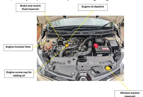
The window washer cap usually has a symbol of a window with water squirting either side.
