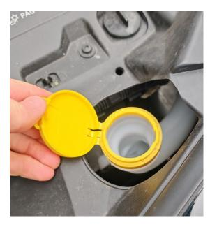
Add either the washer fluid, water or mixture of both into the filler cap. There is no minimum or maximum for this. Just fill it until it is full.
