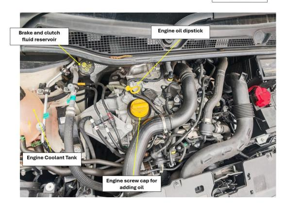
The next pictures show the steps to check the oil level using the dipstick.
