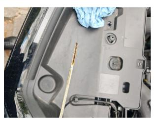
Once clean, replace the dipstick fully into its tube and pull it out. You should be able to see where the oil level is. The ideal oil level will be just under the maximum
