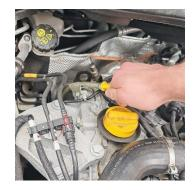
If it is too low, you need to add the right type of oil into your engine. Remove the screw cap on the top of your engine like the one below.
