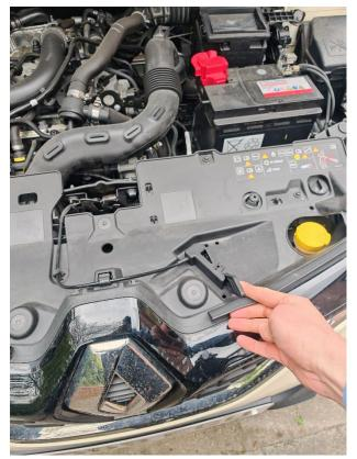
On this Renault, the lever is here. Push it to the left and lift the bonnet. The bonnet will either stay up on its own or there will be a little prop which you will have to find and prop the bonnet up.
