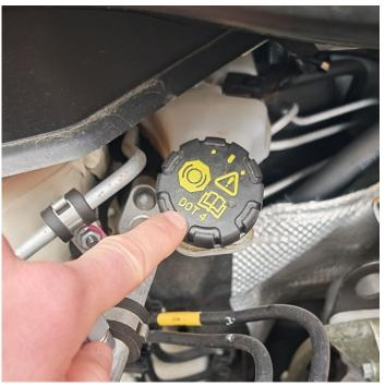
This is an easy one to check. Simply look at the side of the reservoir and it will have a minimum and maximum line. Ensure your fluid is just under the maximum line.
